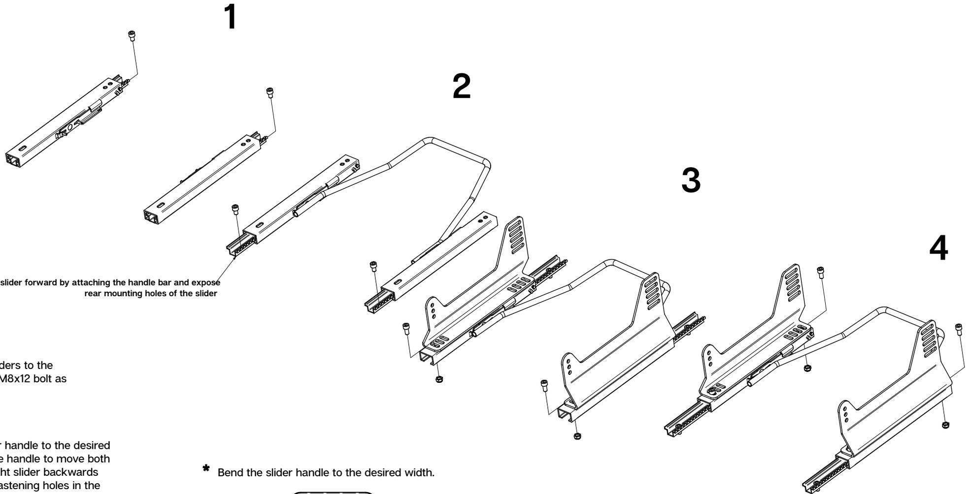
Move slider forward by attaching the handle bar and expose rear mounting holes of the slider
