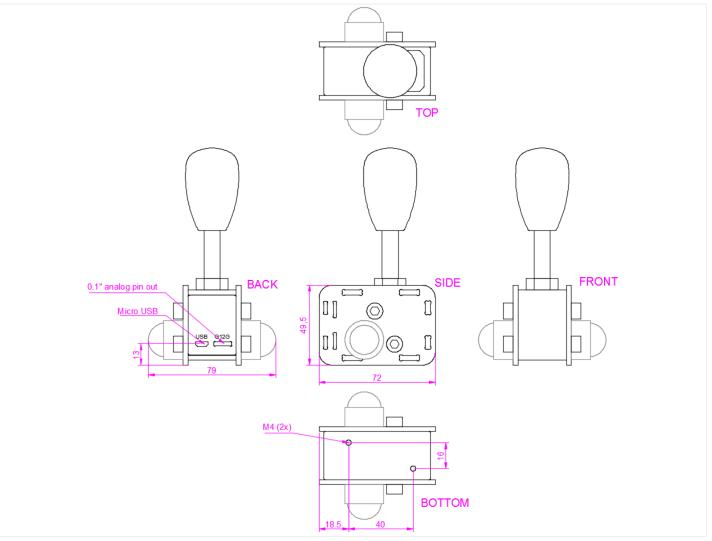
The shifter can be mounted to any flat surface using the 2 M4 bolt holes at the bottom of the unit.
