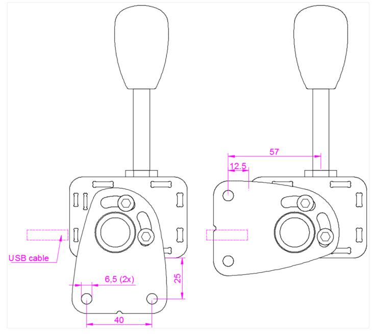
The supplied mounting plate can be mounted to the side of the shifter. By flipping the mounting plate, you can either mount it to a structure (such as an aluminium profile) below or in front of the shifter.
