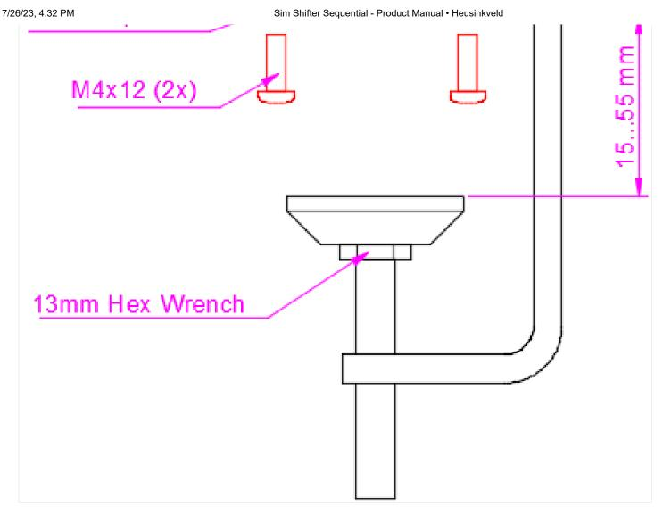
A table clamp is supplied with every shifter. This allows you to connect the shifter to a flat surface below the shifter unit.
