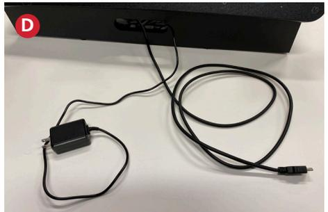
**D:** Run both the other end of the HDMI cable and power cable through the back of the cabinet. Plug the HDMI into your TV and power plug into an outlet.
