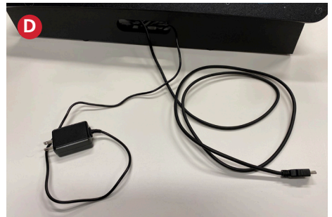
D: Run both the other end of the HDMI cable and power cable through the back of the cabinet. Plug the HDMI into your TV and power plug into an outlet.
