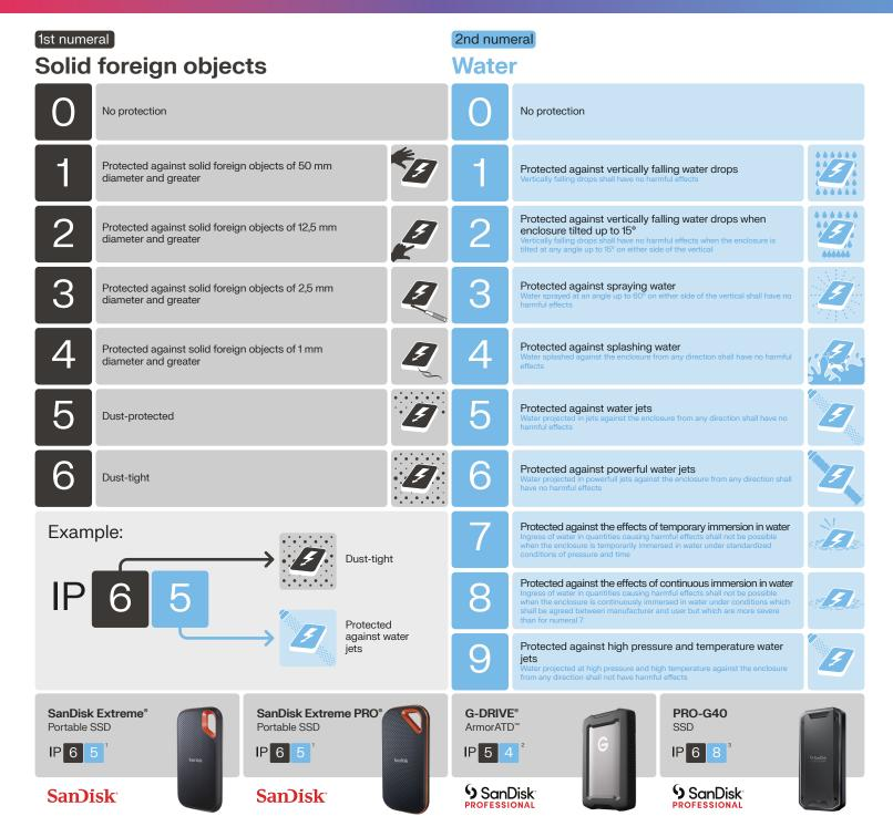
1. Based on internal testing. IPEC 60529 IP 65: Tested to withstand water flow (30 kPa) at 3 min.; limited dust contact does not interfere with operation. Must be clean and dry before use. 2. IEC 60529 IP54: Based on internal testing. Tested to withstand water splashing against the enclosure; limited dust contact does not interfere with operation. Must be clean and dry before use. 3. Based on internal testing.
